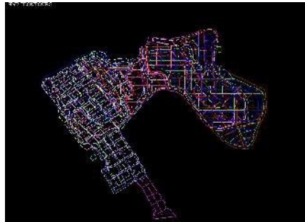
Heap contours imported from an AutoCAD file to simulate an existing copper heap leach project.
